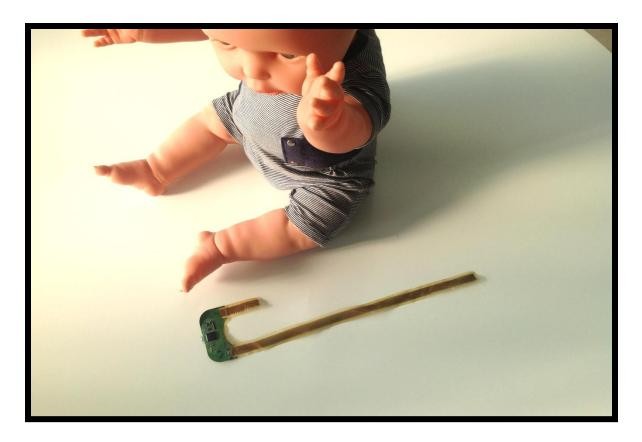
SIDS monitoring as lead application for streatchable sensors & electronics in wearables.
